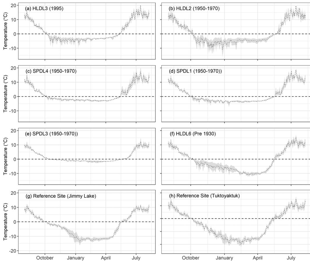
**FIGURE 4** Temperature at 0.1 m below the ground surface at six drained lakes and two reference sites in the Tuktoyaktuk Coastlands. The dotted line shows the mean daily temperature from 2013 to 2017 and the shaded area represents the 95% confidence interval of the daily mean. HLDL and SPDL are abbreviations for Husky Lakes Drained Lake and Swimming Point Drained Lake, respectively. Note the changes in the y-axis scale between (a)–(f) and (g)–(h)
