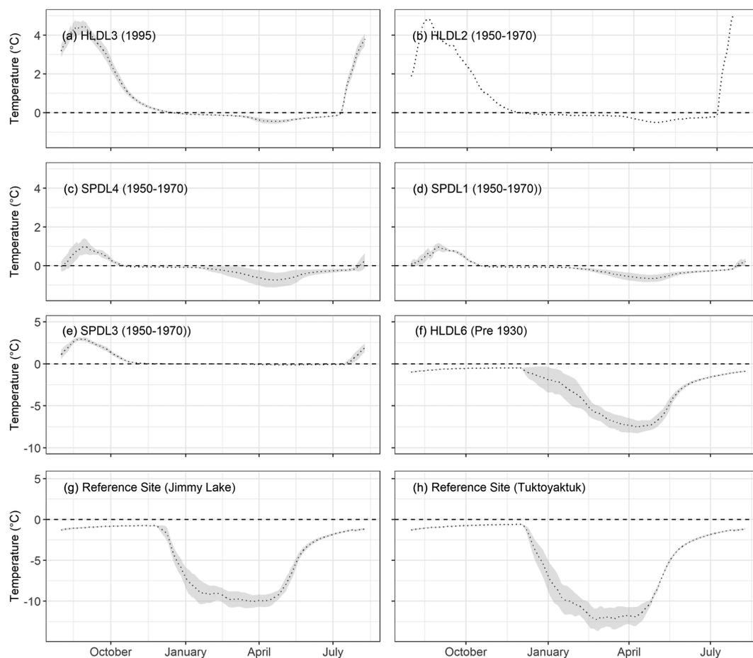
**FIGURE 5** Temperature at 1 m below the ground surface at six drained lakes and two reference sites in the Tuktoyaktuk coastlands. The dotted line shows the mean daily temperature from 2013 to 2017 and the shaded area represents the 95% confidence interval of the daily mean. HLDL and SPDL are abbreviations for Husky Lakes Drained Lake and Swimming Point Drained Lake, respectively. Note the changes in the y-axis scale between (a)–(d), (e)–(f), and (g)–(h)
