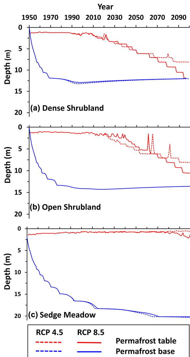
**FIGURE 6** Modeled permafrost conditions (1950–2100) in three drainage scenarios: (a) dense shrubland, (b) open shrubland, and (c) sedge meadow. The red lines show the depth to the top of permafrost and the blue lines show the depth to the base of permafrost. Model runs using climate data from RCP 4.5 (2020–2100) are shown as dashed lines and model runs using RCP 8.5 data are shown as solid lines [Colour figure can be viewed at [wileyonlinelibrary.com](https://onlinelibrary.wiley.com)]
